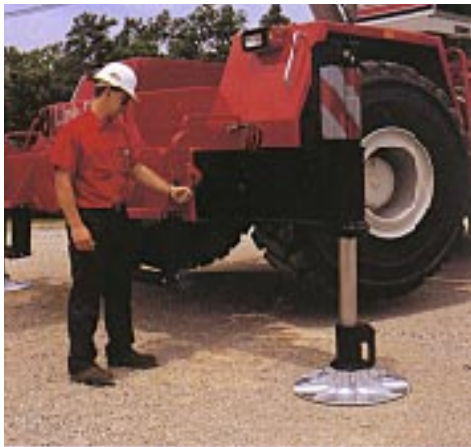
Fully Extended Outriggers 22' 0" (6.71 m) spread
