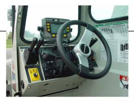
**Operator cab** Hydraulic proportional joystick controls, automotive dash layout, tilt steering wheel, and suspension seat enhances operator comfort and ease of use.
