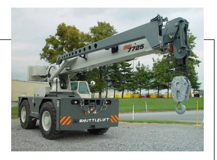
The reach and capacity to get the job done A 5,1 m (17 ft) swingaway extension added to the 21,6 m (71 ft) main boom provides an impressive 28,9 m (95 ft) tip height with a capacity of 2268 kg (5000 lb). A galvanized down-haul ball is included with the extension.
