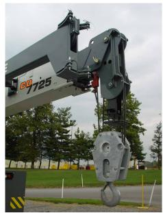
Hook block A galvanized coated hook block is provided as standard to help eliminate rusting of this important crane component.
