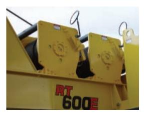
The RT600E uses a 12,250 lbs. pinned-on counterweight. Cable power is provided through model HP30A grooved drum hoists with 16,800 lbs. permissible line pull. Max line speed is 588 fpm. Both the main and optional auxiliary hoists have cable capacity up to 694 ft.
